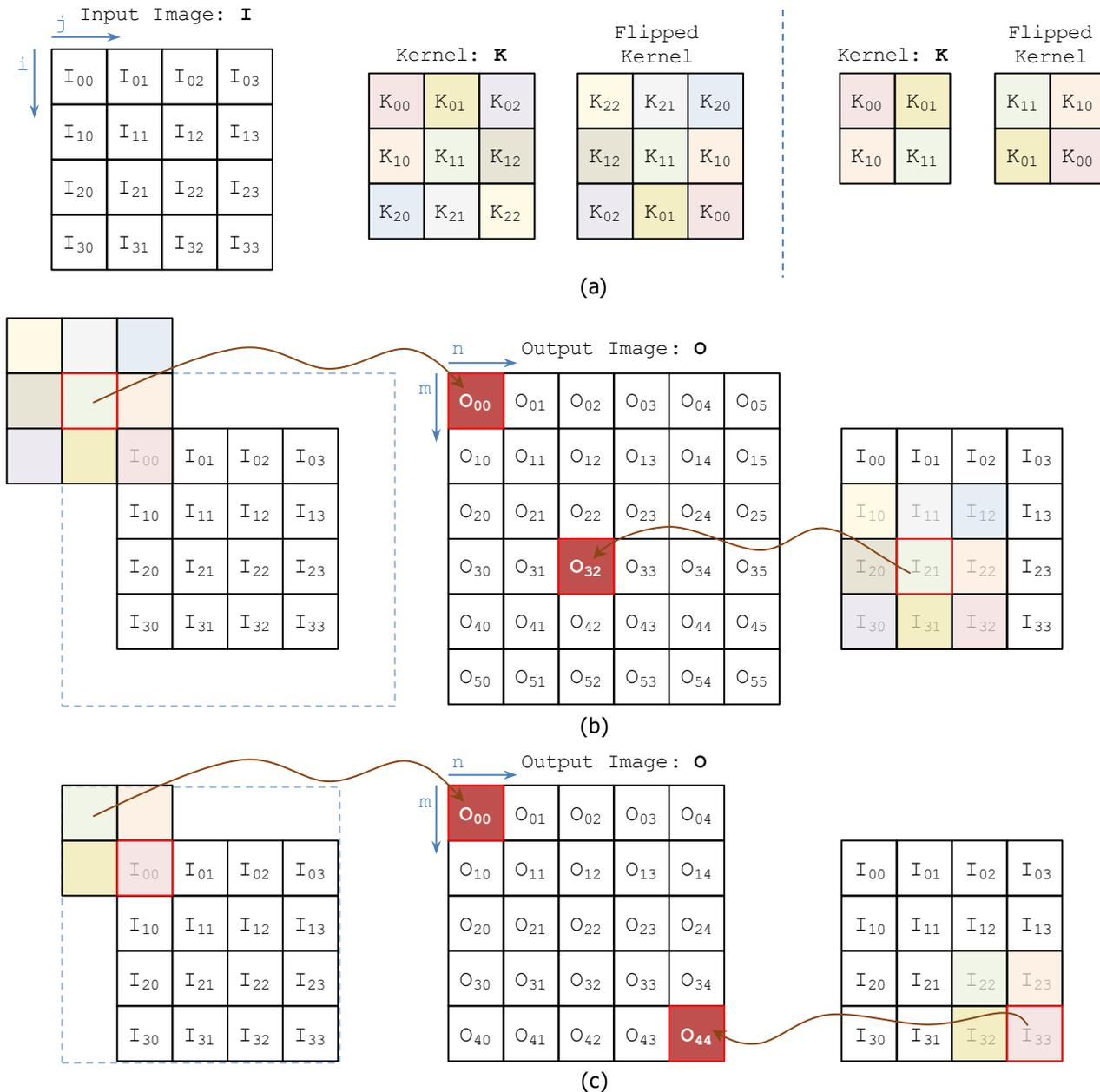
Figure 3. 2D convolution. (a) Input image:  $I(4 \times 4)$ . Kernels:  $3 \times 3$  and  $2 \times 2$ . (b) Convolution with  $3 \times 3$  kernel. Output Image:  $O(6 \times 6)$ . (c) Convolution with  $2 \times 2$  kernel. Output image:  $O(5 \times 5)$ .
